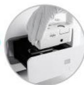
**Step 4:** The cartridge is inserted into one of the available instruments, which will subsequently execute the appropriate test protocol. After completion of the test, results are displayed on the console.
