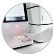
**Step 2:** The patient sample is linked to the cartridge by scanning the barcode of the cartridge. The console automatically recognizes which test the user intends to perform.
