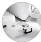
**Step 3:** The patient sample is added into the cartridge. By closing the lid, the cartridge is hermetically sealed to prevent contamination of the instrument or laboratory.
